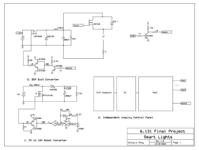
The circuit design includes a boost converter, a DCM buck converter, and a control panel (a PSoC) that can be interacted with through a MIDI keyboard.
