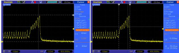
These current spikes (actually made of a series of shorter spikes due to differing turn-on speeds of the MOSFETs) are within specifications for the LEDs. The spikes are less than 100 mA - the maximum current for the LEDs, they are less than 0.1 ms long, and they occur for far less than
