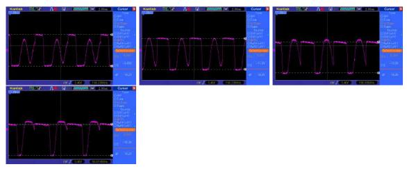
The buck converter additionally performs well under the target conditions, with each LED turning on and off at a PWM rate of 100 Hz. The resolution for this PWM is 0 to 127. To evaluate performance, a test pattern A of 0, 20, 40, 60, 80, 100, and 120 brightness values on the LEDs and a test pattern B with 63 on each LED was used.
