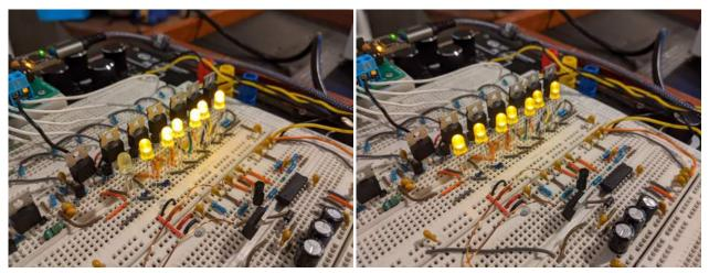
Shown below is the PSoC control panel when in scene program mode; the status LEDs are displaying a new pattern being programmed.
