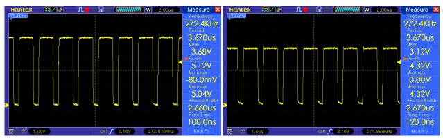
As determined by the oscilloscope, the duty cycle achieved is roughly  $\frac{2.670 \,\mu\text{s}}{3.670 \,\mu\text{s}} = 0.728$ .
